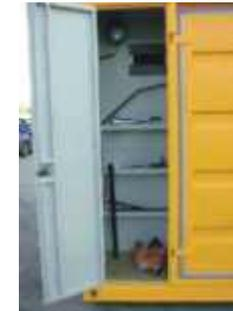
In the left front part is the tool compartment for special tools leaving even enough space to store spare and wearing parts.
